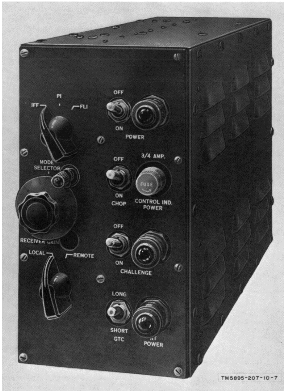
Figure 5. Coder-Control, Interrogator Set KY-97B/TPX, front panel.
